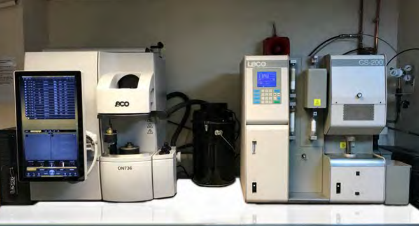
Combustion Analysis to measure ultra low levels of carbon, nitrogen and oxygen
