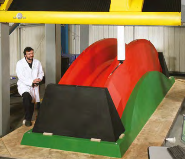
Large scale pattern inspection
