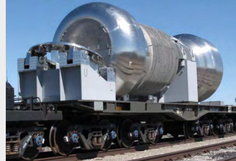
Nuclear flask for the defueling of submarines, manufactured to ASME codes
