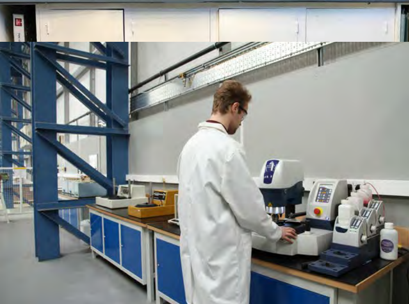
Metallographic Polishing & Chemical Etching of Specimens
