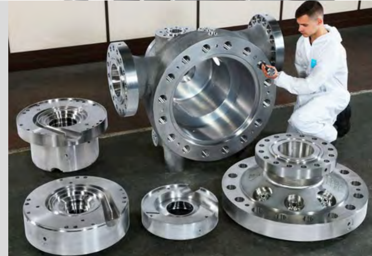
Pump and Volute Castings in 316 Stainless Steel
