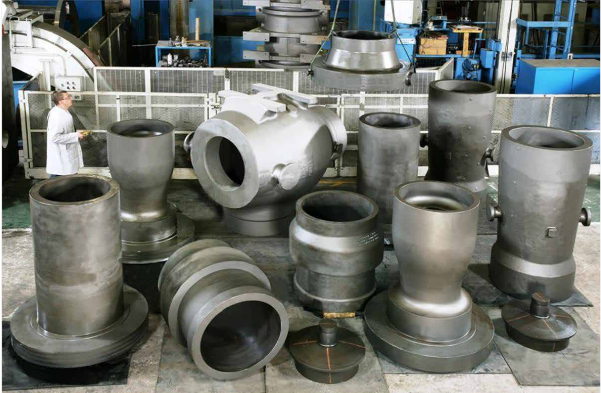
9.5% Cr Steel Machined castings for a 800MW Power Station in India Produced by Goodwin Steel Castings Ltd
