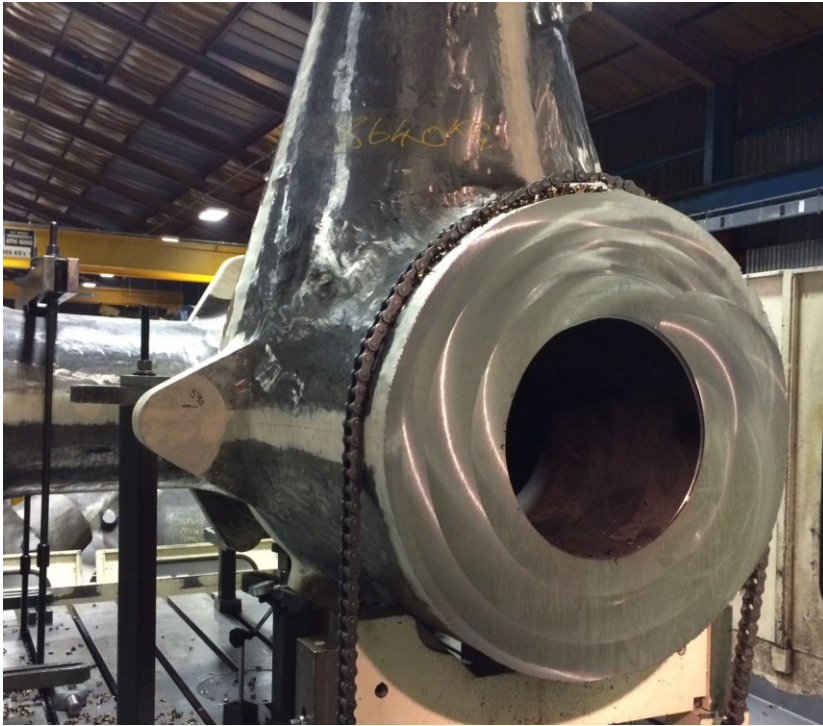
Figure 2 – 8,640 Kg MarBN Steel steam valve demonstration casting manufactured within the UK INMAP project (4) (heaviest section 200mm)
