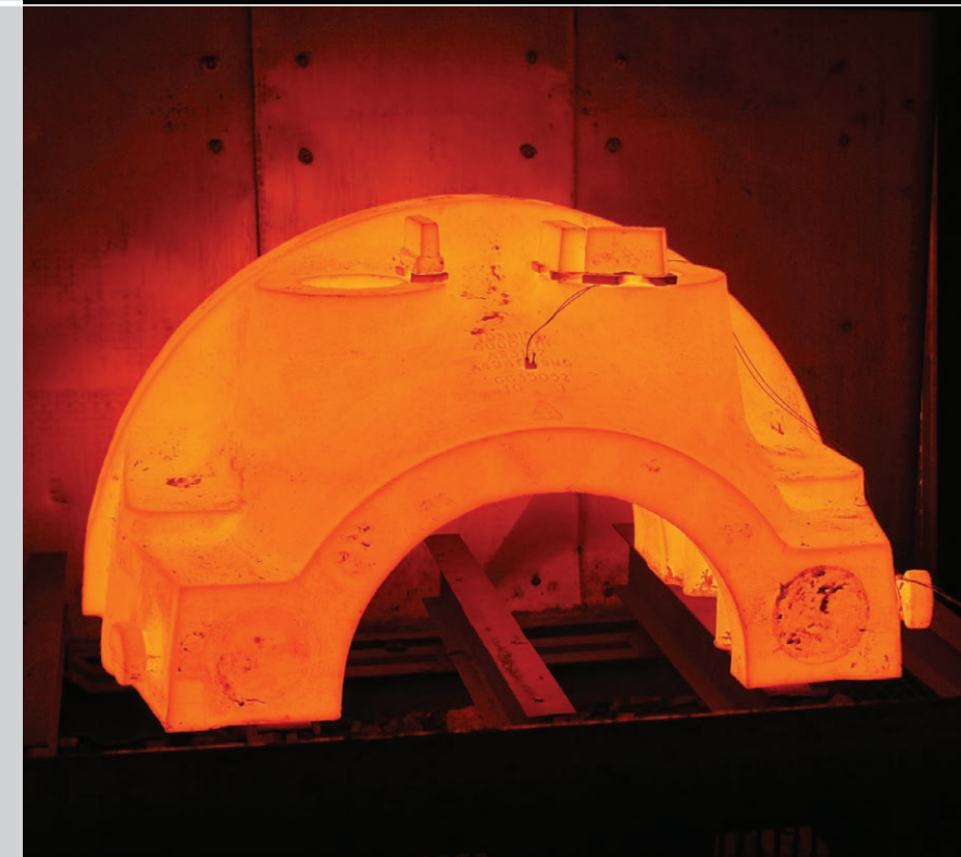
10,500kg Alloy 625 HP Casing during quality heat treatment.
