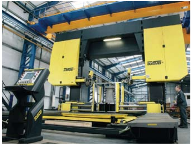
Left: CNC gantry saw with cutting portal of 3m x 3m and 7m travel Main pic: Suite of 12" and 16" Super Duplex valve bodies
