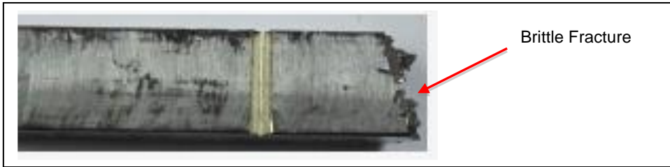
Fig 15: Shows an impact specimen from the standard cast chemistry for Alloy 740H. The specimen has broken outside of the notch and is showing brittle fracture characteristics. This was caused by cracked carbide precipitates at the grain boundaries. (Results 10Joules) –The tensile specimens showed the same problem with fractures taking place outside of the gauge length.
