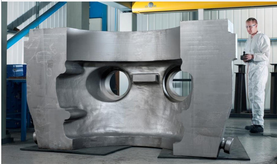
Fig 2: 10,500Kg Alloy 625 HP Casing manufactured by Goodwin 2011-2012 Supplied in the proof machined condition with section Sizes up to 435mm Goodwin have also produced an 11,000kg HP Casing
