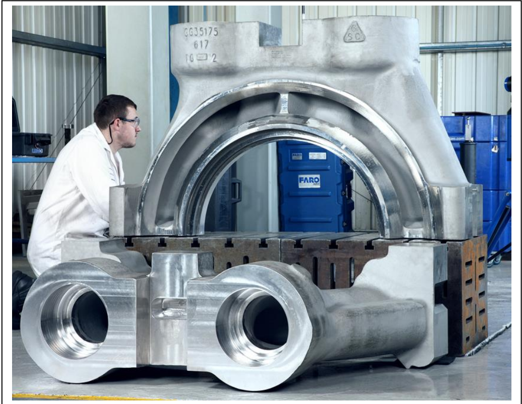
Fig 5: Nozzle Box Castings: Alloy 617 Mod and Alloy 625 Net Weight: 1,800Kg – both castings supplied in the proof machined condition: Section size up to 300mm prior to machining
