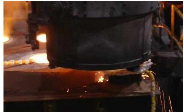
This system seals the ladle stream from air, and therefore prevents oxidation. Argon is also purged into the mould both before and during the pouring operation.
