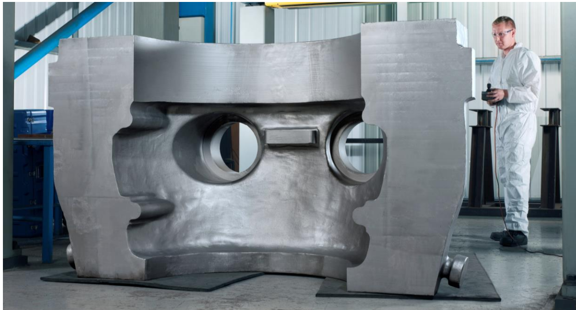
10,500kg Alloy 625 HP Casing manufactured by Goodwin 2011-2012 Supplied in the proof machined condition with section sizes up to 435mm
